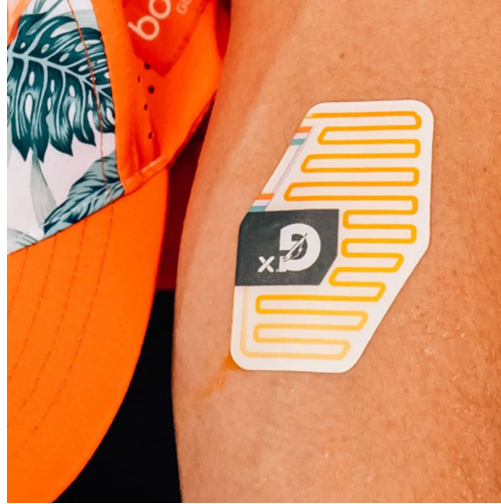
Colorimetric reagents in microfluidic patch Epicore Biosystems Gx
